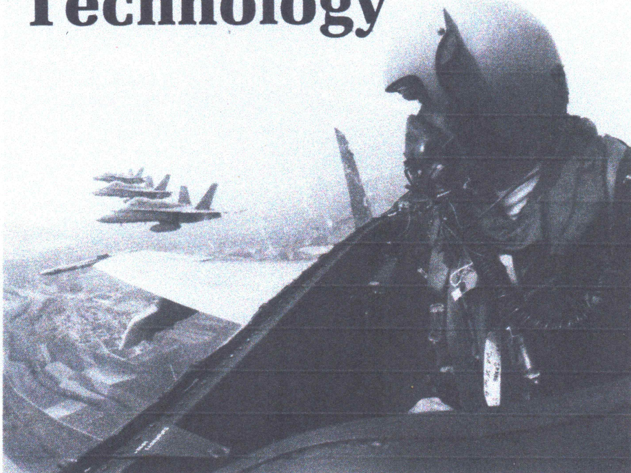
CF-188 Hornets of Canada's 409 Sqn, based in Germany: Some of the paraphernalia of flight safety equipment (helmet, oxygen mask and seat restraints) can be seen. Is the pilot suitably equipped to survive the physical forces imposed on him by his high-tech mount? (Photo: Canadian Armed Forces)
